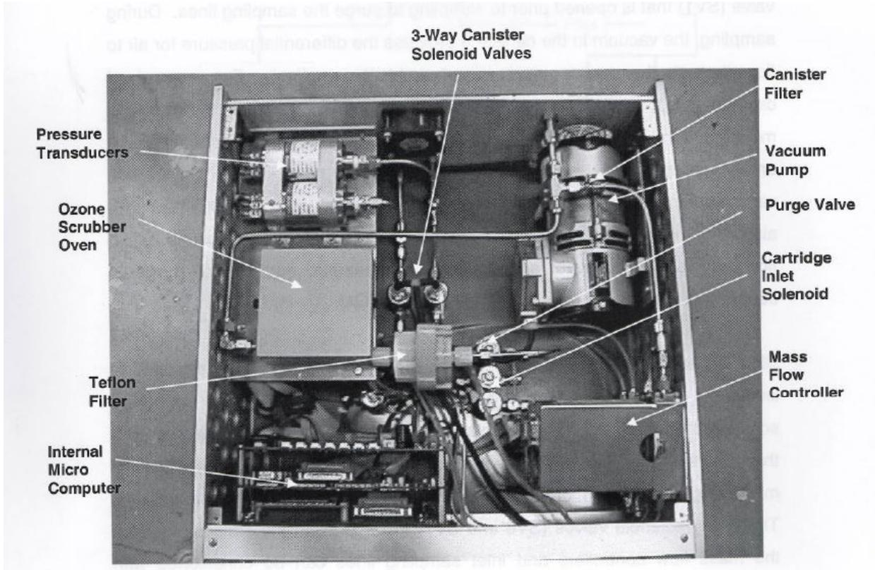
Figure 10. ATEC Model 2200-2 Internal Components
