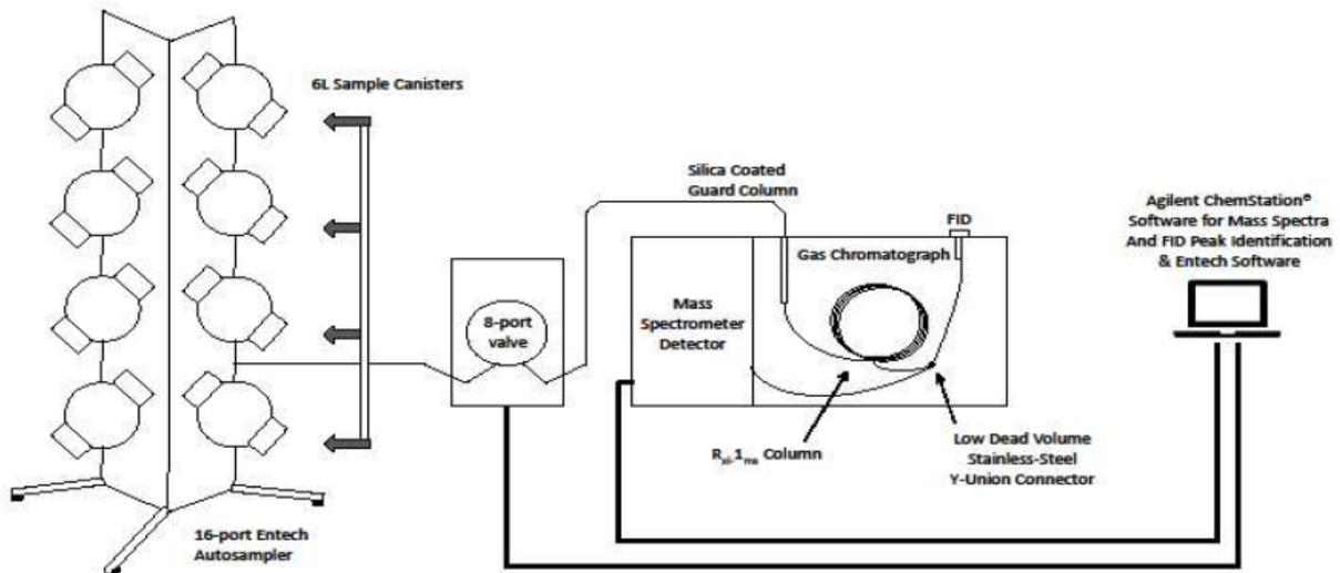
Figure 2. ERG's VOC GC/MS/FID System
