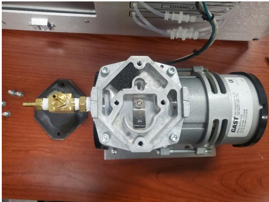
**Figure 8. Pump Inlet and Outlet Valve Replacement**
