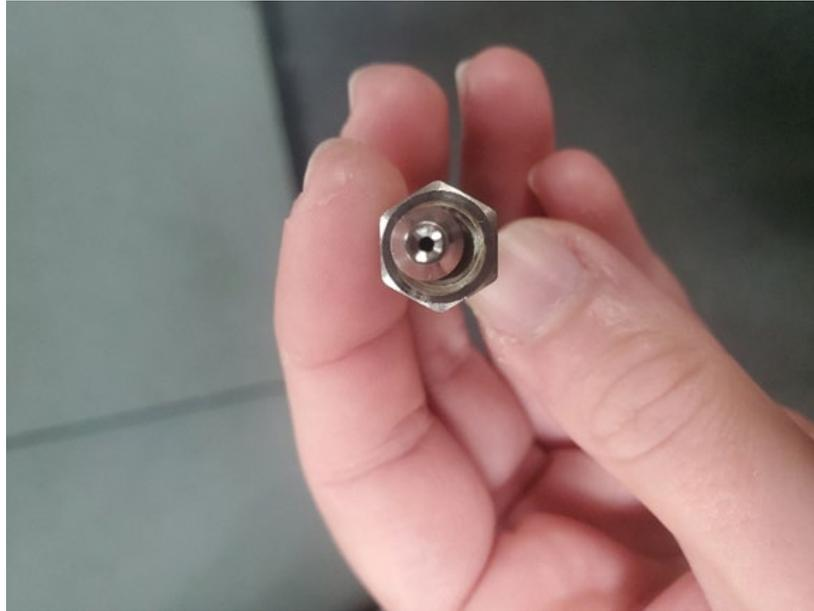
**Figure 9. Acceptable Silco-Line Opening**
