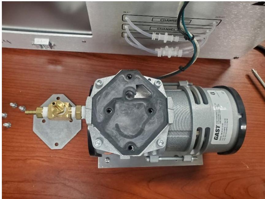
**Figure 7. Pump Gasket Configuration**
