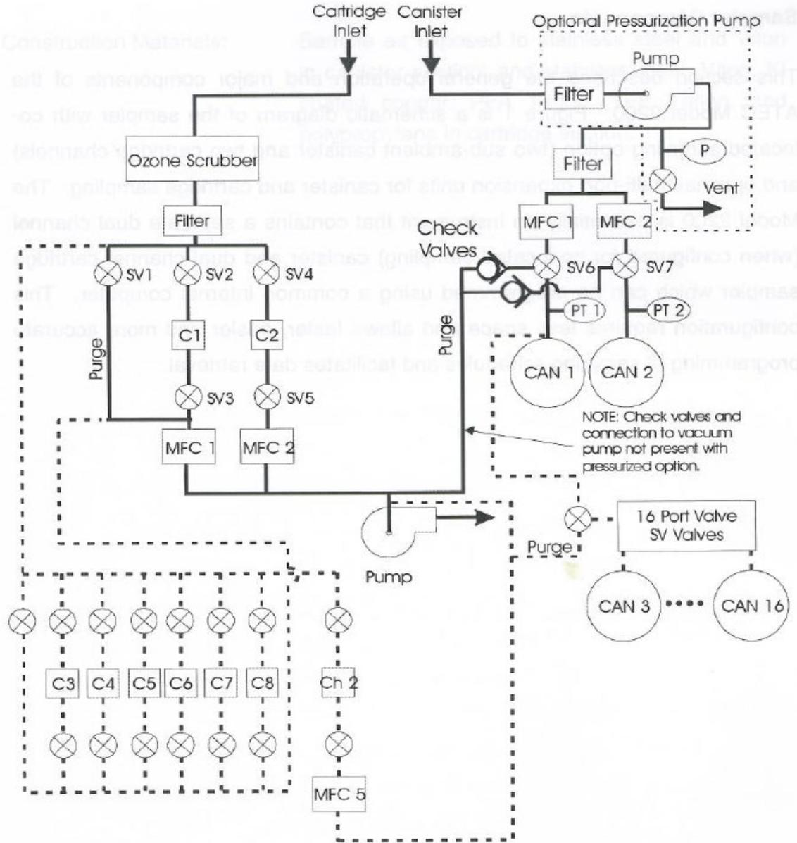
Model 2200 Flow Schematic with Canister and Cartridge Expansions
