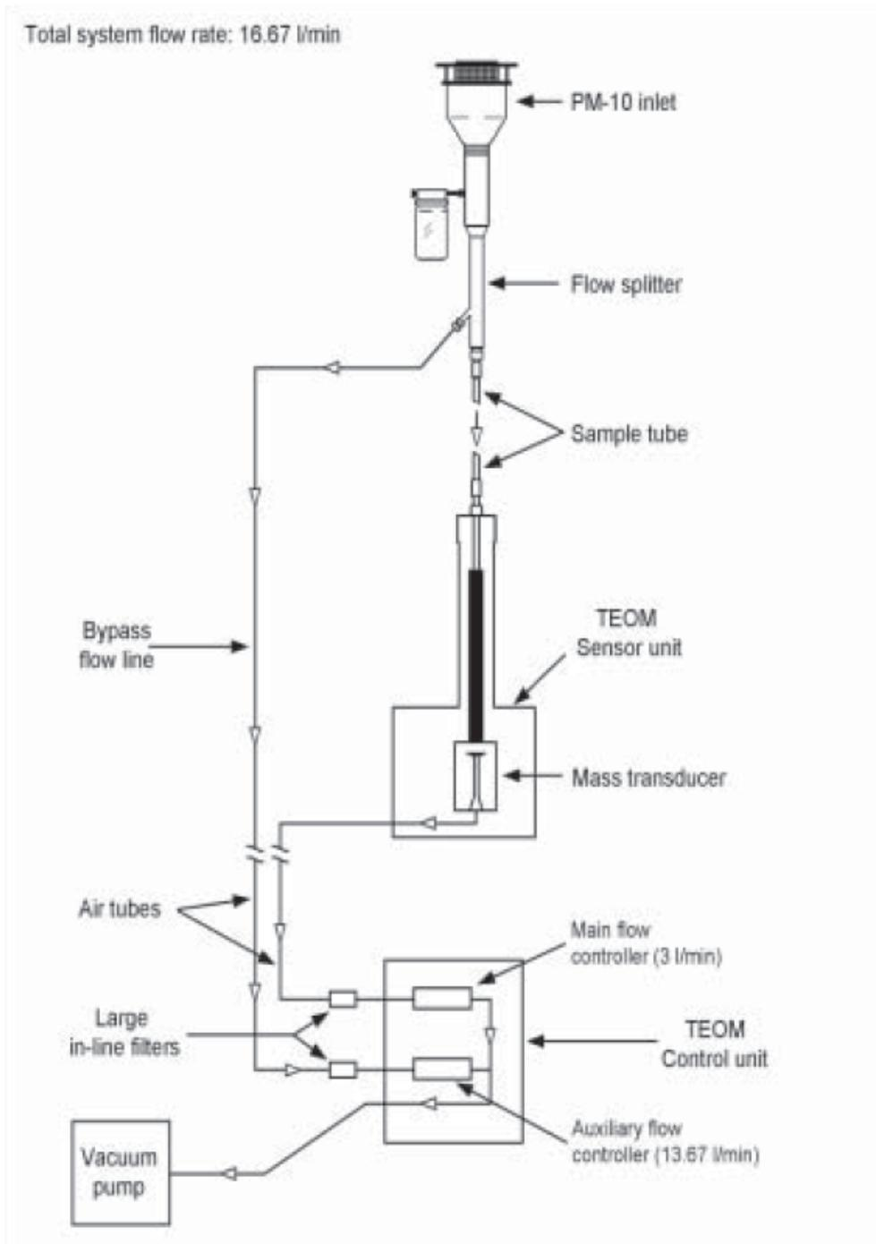
Figure 2 - RP 8500 FDMS/TEOM typical configuration, PM<sub>2.5</sub> sampling.
