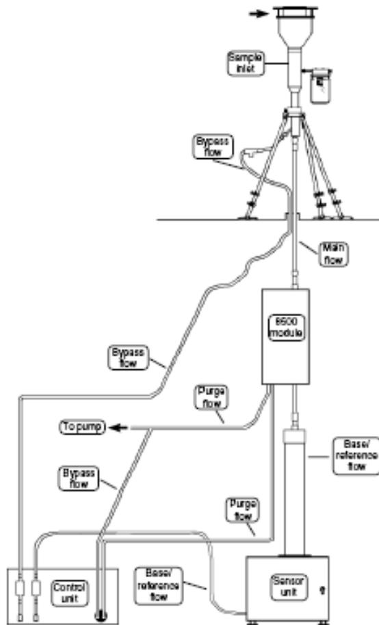
Note: The configuration for PM<sub>2.5</sub> sampling without the FDMS unit is the same as for PM<sub>10</sub> sampling with the addition of a VSCC upstream of the flow splitter. Some additional changes in software settings are also necessary and are discussed below.
