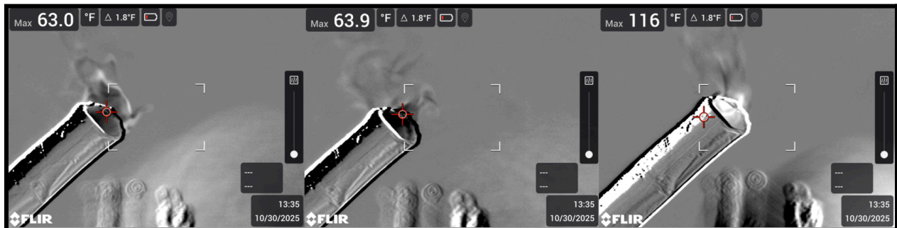
Figure 2: Three frames of FLIR footage showing emissions from the severed pipe on October 30, 2025.
